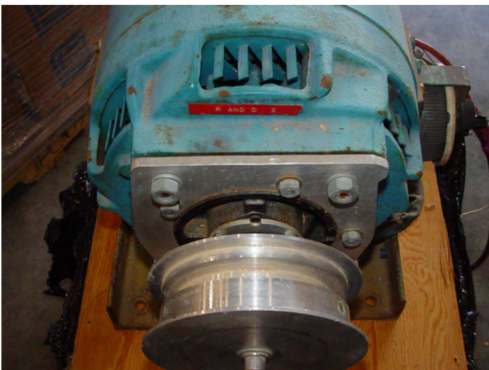
Custom Adapter Flange Added to Front of Motor
